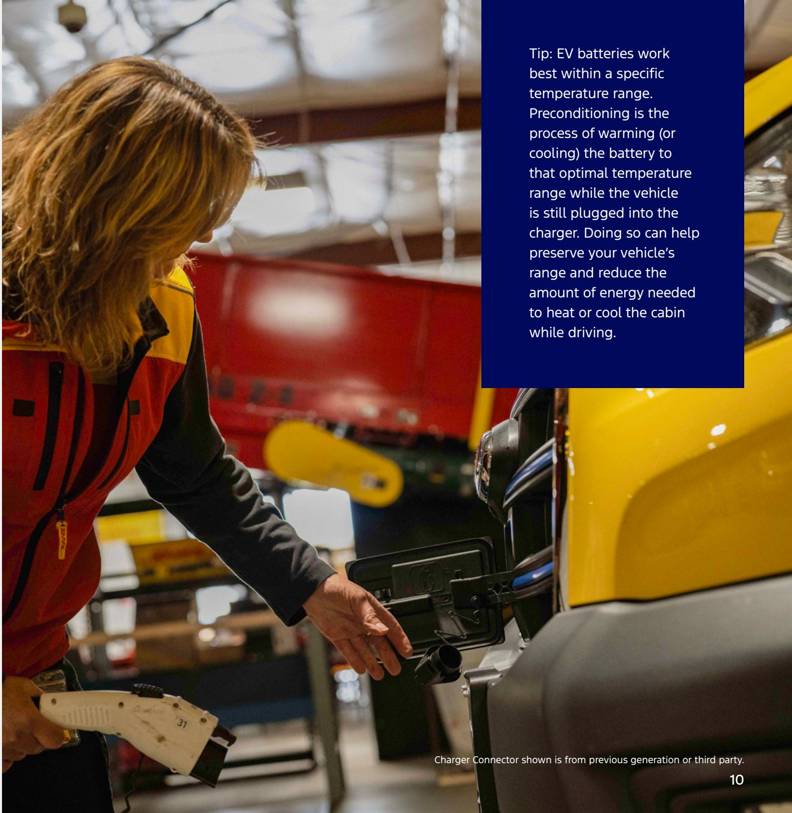
Tip: EV batteries work best within a specific temperature range. Preconditioning is the process of warming (or cooling) the battery to that optimal temperature range while the vehicle is still plugged into the charger. Doing so can help preserve your vehicle's range and reduce the amount of energy needed to heat or cool the cabin while driving.
