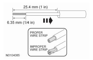
Select the appropriate wire splice for the wires to be spliced from Rotunda Wire Splice Kit 164-R5903.
